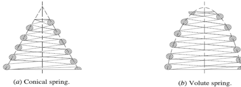
Fig.4.2 Conical and volute springs.
