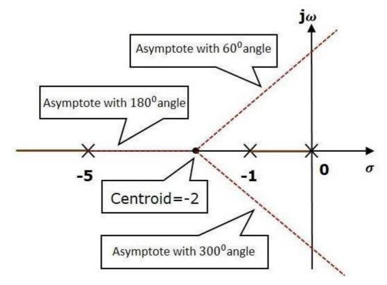
Step 3 – Since two asymptotes have the angles of 600600 and 30003000, two root locus branches intersect the imaginary axis. By using the Routh array method and special case(ii),  $j\sqrt{5} - j\sqrt{5}$ .
