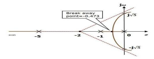
In this way, you can draw the root locus diagram of any control system and observe the movement of poles of the closed loop transfer function.
