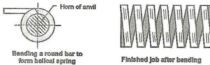
Fig. 3.35 : Bending a round bar to form a helical spring
