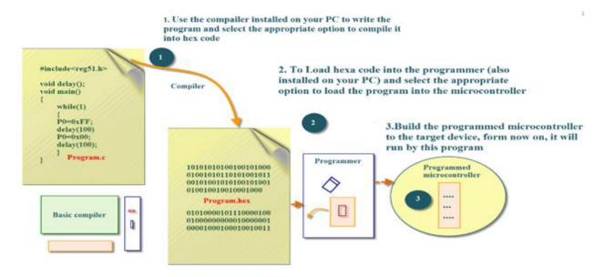
The Embedded C code written in above block diagram is used for blinking the LED connected with Port0 of microcontroller.
