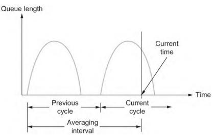
Average queue length is measured over a time interval that includes the last busy + last idle cycle + current busy cycle.
