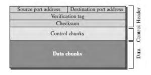
An SCTP packet has a mandatory general header and a set of blocks called chunks.
