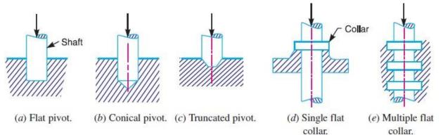
A conical pivot supports a load of 20 kN, the cone angle is 120° and the intensity of normal pressure is not to exceed 0.3 N/mm2. The external diameter is twice the internal diameter. Find the outer and inner radii
