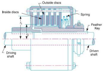
**Example 10.22.** Determine the maximum, minimum and average pressure in plate clutch when the axial force is 4 kN. The inside radius of the contact surface is 50 mm and the outside radius is 100 mm. Assume uniform wear.
