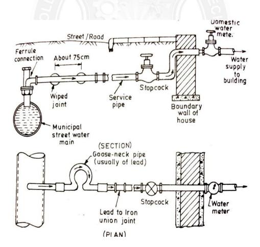
(d) Stop cock - Provided before the water meter in the house. It is housed in a masonry chamber with removable cover and fixed in the street close to the boundary wall.
