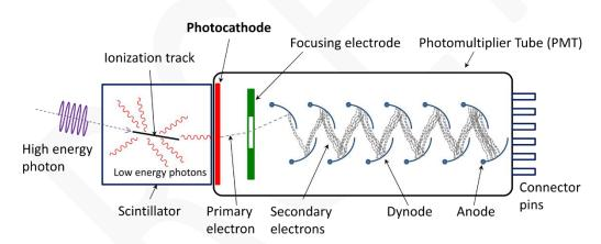
A scintillation detector is made up of a scintillator and photodetector. It consists of a scintillator which generates photons in response to incident radiation, a sensitive photodetector (usually a photomultiplier tube (PMT), a charge-coupled device (CCD) camera, or a photodiode), which converts the light to electrical signal and electronics to process this signal.
