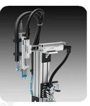
A popular application is to pick and place small components into an assembly, maybe from avibratory bowl feeder to an assembly fixture.
