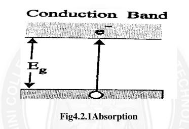
For extrinsic semiconductor, electron transition is between donor and conduction band in n type semiconductor and for p type it is between acceptor and valence band
