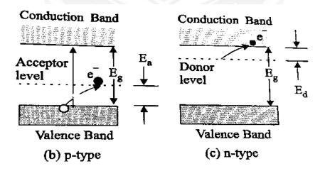
Fig 4.2.2.Absorption & emission in semiconductors
