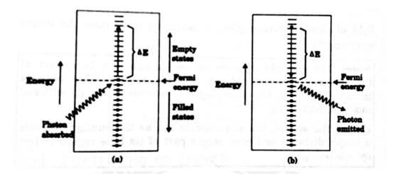
Fig 4.2.3. Absorption and emission in metals
