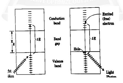
Fig 4.2.4. Absorption and emission in insulators
