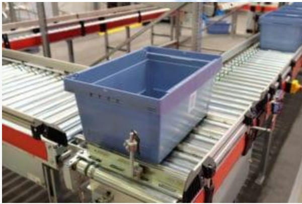
Right Angle Transfer Conveyor
