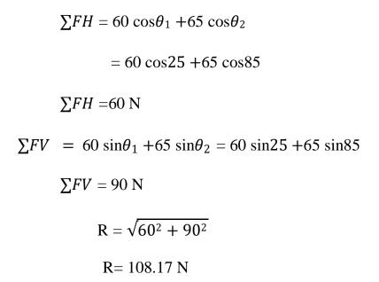
Two wires are attached to a bolt in a foundation as shown in fig. below.
