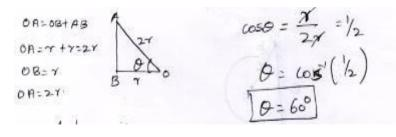
Apply  $\Sigma FH=0$ R<sub>B</sub>-T<sub>CA</sub> cos 60 = 0 -----(1)  $\Sigma FV=0$ T<sub>CA</sub> sin 60- w=0 -----(2)
