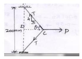
15. Two cables are tied together at c and are loaded as shown in fig below.Determine the tension in the cable AC and BC
