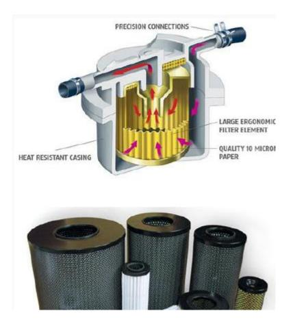
Further to remove the fine particles and abrasive material in the fuel, secondary filter is used which is made of fine pores and it is placed after the fuel feed pump. These smallest impurities are retained to protect the extremely sensitive parts like fuel pump and injectors to get damaged. These filters are generally made of two sections/stages in which first stage is made of cloth and second is of paper through which the fuel passes to leave impurities behind in the fuel line.
