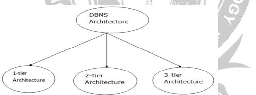
Database architecture can be seen as a single tier or multi-tier. But logically, database architecture is of two types like: **2-tier architecture** and **3-tier architecture**.
