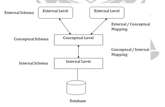
**1.The internal level** – has an internal schema which describes the physical storage structure of the database. Uses a physical data model and describes the complete details of data storage and access paths for the database.
