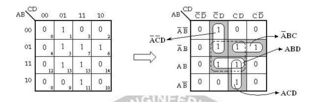
In the above K-map, the cells 5, 7, 13 and 15 can be grouped to form a quadas indicated by the dotted lines. In order to group the remaining 1's, four pairs have to be formed. However, all the four 1's covered by the quad are also covered by the pairs. So, the quad in the above k-map is redundant.
