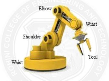
The *Anatomy* of Industrial Robots deals with the assembling of outer components of a robot such as wrist, arm, and body. Before jumping into Robot Configurations, here are some of the key facts about robot anatomy.
