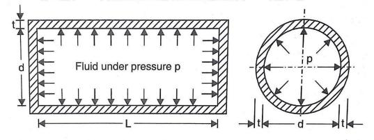
One of the internal pressure p, the cylindrical vessel may fail by splitting up in any one of the two ways.
