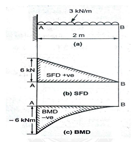
**Bending moment Calculation:** [Sum of (Vertical force x Distance of load acting from required section)]
