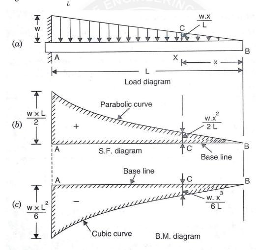
The resultant force acting on the right portion acting downward is considered positive. The shear force at the section X at a distance x from free end is given by
