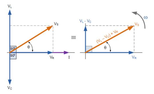
We can see from the phasor diagram on the right hand side above that the voltage vectors produce a rectangular triangle, comprising of hypotenuse  $V_S$ , horizontal axis  $V_R$  and vertical axis  $V_L - V_C$  Hopefully you will notice then, that this forms our old favourite the Voltage Triangle and we can therefore use Pythagoras's theorem on this voltage triangle to mathematically obtain the value of  $V_S$  as shown.
