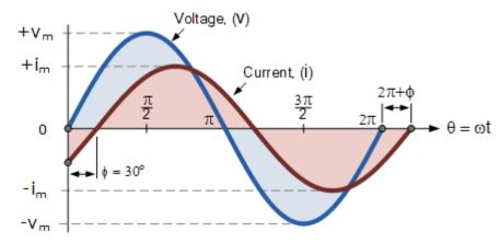
The voltage waveform above starts at zero along the horizontal reference axis, but at that same instant of time the current waveform is still negative in value and does not cross this reference axis until 30° later. Then there exists a Phase difference between the two waveforms as the current cross the horizontal reference axis reaching its maximum peak and zero values after the voltage waveform.
