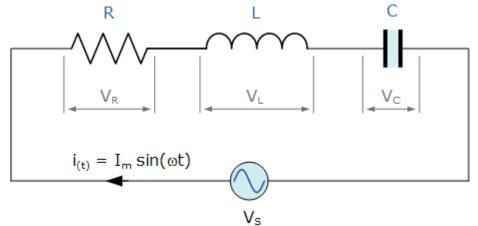
In a pure ohmic resistor the voltage waveforms are "in-phase" with the current. In a pure inductance the voltage waveform "leads" the current by 90°, giving us the expression of: ELI. In a pure capacitance the voltage waveform "lags" the current by 90°, giving us the expression of: ICE.
