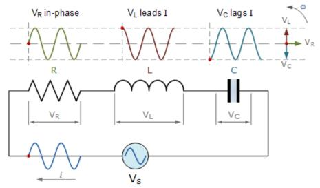
The amplitude of the source voltage across all three components in a series RLC circuit is made up of the three individual component voltages,  $V_R$ ,  $V_L$  and  $V_C$  with the current common to all three components. The vector diagrams will therefore have the current vector as their reference with the three voltage vectors being plotted with respect to this reference as shown below.
