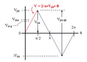
When plotted as voltage (V) as a function of phase ( $\theta$ ), a triangle wave looks similar to the figure to the above. The waveform repeats every  $2\pi$  radians (360°), and is symmetrical about the voltage axis (when no DC offset is present). Voltage and current exhibiting cyclic behavior is referred to as alternating; i.e., alternating current (AC). One full cycle is shown here. The basic equation for a triangle wave is as follows:
