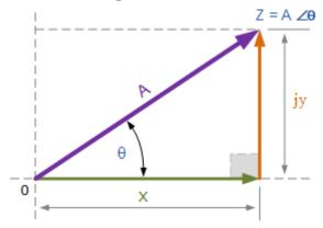
As the polar representation of a point is based around the triangular form, we can use simple geometry of the triangle and especially trigonometry and Pythagoras's Theorem on triangles to find both the magnitude and the angle of the complex number. As we remember from school, trigonometry deals with the relationship between the sides and the angles of triangles so we can describe the relationships between the sides as:
