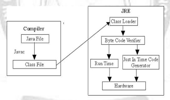
**Class Loader**: is the subsystem of JVM that is used to load class files.
