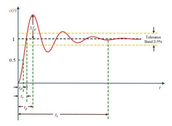
All the time domain specifications are represented in this figure. The response up to the settling time is known as transient response and the response after the settling time is known as steady state response.
