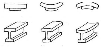
Required Shape of Casting Distorted Casting Cambered Pattern
