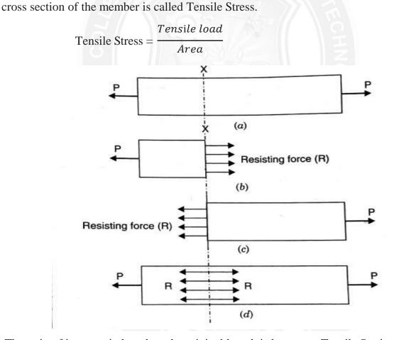
The ratio of increase in length to the original length is known as Tensile Strain
