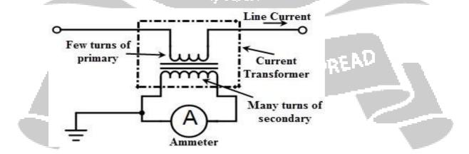
Primary of C.T. is having very few turns. Sometimes bar primary is also used. Primary is connected in series with the power circuit. Therefore, sometimes it also called series transformer.
