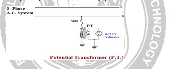
Primary of P.T. is having large no. of turns. Primary is connected across the line (generally between on line and earth). Hence, sometimes it is also called the parallel transformer.
