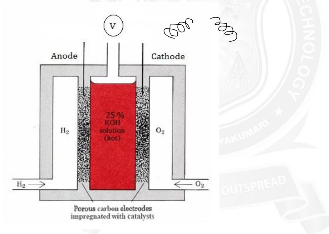
Fig:1-Hydrogen-oxygen fuel cell
