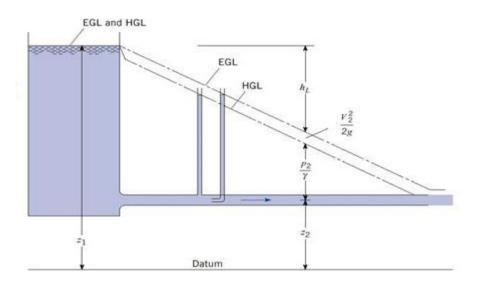
Hydraulic gradient and energy lines are displayed in figure.
