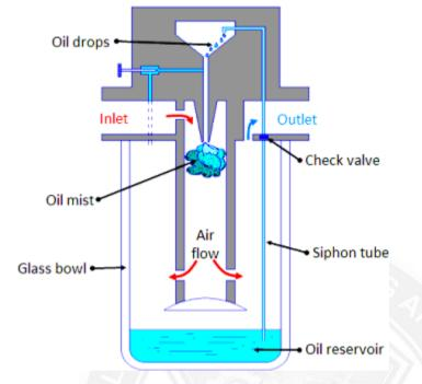
The compressed air is first filtered and then passed through a lubricator in order to form a mist of oil and air to provide lubrication to the mating components. Figure
