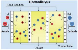
Water is handed between a negative electrode and a high-quality electrode. Ion exchange membranes permit solely high-quality ions to transfer toward the negative electrode from the feedwater and negative ions to the positive electrode.
