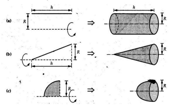
Bodies of revolution are obtained by revolving areas about an axis. A few examples are shown in Fig.
