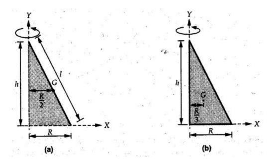
The volume of cone is generated by revolving a triangle as shown in Fig. about Y-axis.
