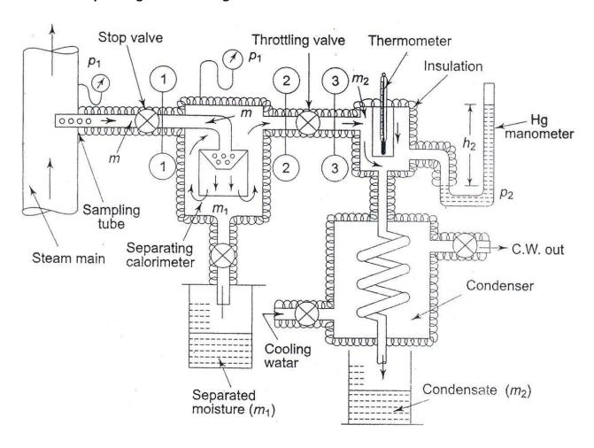
When the steam is very wet and the pressure after throttling is not low enough to take the steam to the superheated region, then a combined separating and throttling calorimeter is used for the measurement of quality.
