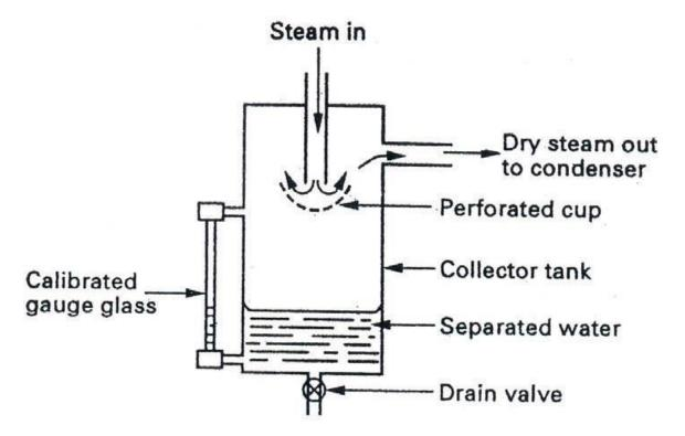
The wet steam enters at the top from the main steam pipe through holes in the sampling pipe facing up stream which should be as far as possible downstream from elbows and valves to ensure representative sample of steam when in operation the wet steam entering passes down the central passage and undergoes a sudden reversal of direction of motion when strikes perforated cup.
