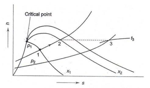
Separating and throttling processes on h-s plot
