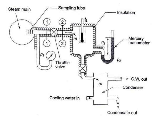
In the throttling calorimeter, a sample of wet steam of mass m and at pressure P1 is taken from the steam main through a perforated sampling tube. Then it is throttled by the partially-opened valve (or orifice) to a pressure P2 measured by mercury manometer, and temperature t2, so that after throttling the steam is in the superheated region.
