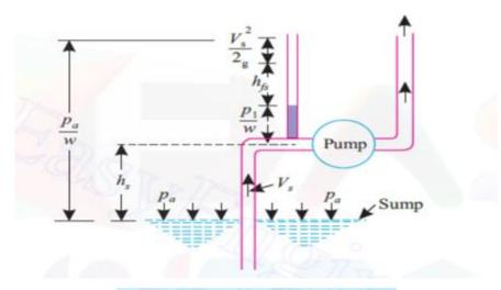
Pressure balance at pump section.
