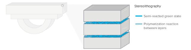
Isotropy has both mechanical and optical benefits. Isotropic parts are ideal for engineering prototyping applications, since they reflect the range of properties associated with common injection-molded thermoplastics and don't suffer from delamination or surface porosity. The chemical bonding process and the lack of visible layer lines inside the parts allows for printing of optically clear parts.
