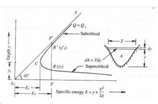
2.  $E = Constant = E1 \rightarrow E1 = f(y,Q)$  Variation of the discharge with the water depth at across-section for a given specific energy E1.
