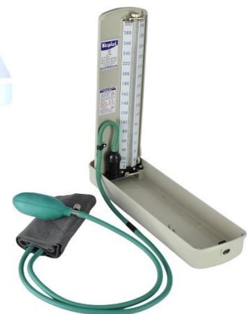
Fig. 4.2 Mercury manometer and pressure cuff
