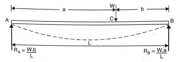
The above equation of B.M. holds good for the values of x between 0 and 'a'. The bending moment at any section between C and B at a distance x from A is given by,
