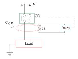
Single Phase Residual Current ELCB. The polarity of the phase winding and neutral winding on the core is so chosen that, in normal condition mmf of one winding opposes that of another.
