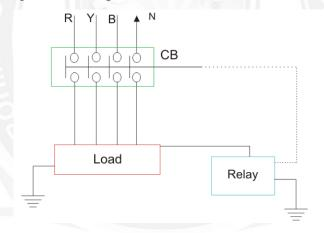
If the voltage difference crosses, a predetermined limit, the current through the relay becomes sufficient to actuate the relay for tripping the associated circuit breaker to disconnect the power supply to the equipment.
