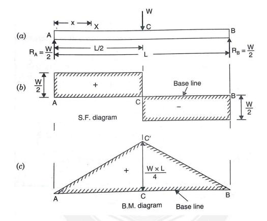
First to find the reaction force at A and B as  $R_A$  and  $R_B$  by the two steps are followed. Step1: Take moment about A = 0 »  $R_B \ge L - W \ge \frac{L}{2} = 0 \gg R_B = \frac{W}{2}$
