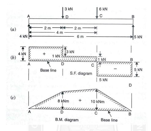
**Bending moment Calculation:** [Sum of (Vertical force x Distance of load acting from required section)]
