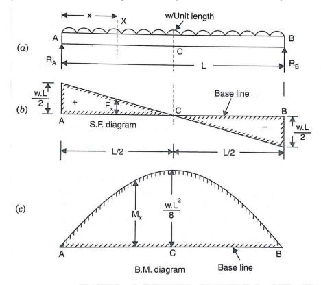
First to find the reaction force at A and B as  $R_A$  and  $R_B$  by the two steps are followed. Step1: Take moment about  $A = 0 \gg R_B \ge L - w \cdot L \ge 2 = 0 \gg R_B = \frac{WL}{2}$ Step2: Sum of upward force = Sum of downward force  $\gg R_A + R_B = W \cdot L$
