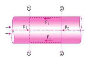
Consider a uniform horizontal pipe having steady flow. Let 1-1, 2-2 are two sections of pipe.
