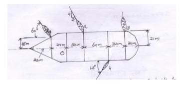
(ii) Determine a single equivalent force and its location along the longitudinal axis of the ship
