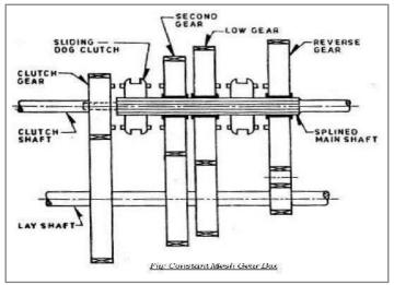
provided on the main shaft- one between the clutch gear and the second gear, and the other between the first gear and reverse gear. The main shaft is splined and all the gears are free on it. Dog clutch can slide on the shaft and rotates with it. All the gears on the countershaft are rigidly fixed with it.
