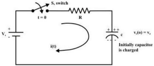
The switch 'S' is closed at time 't=0' It is assumed that the capacitor is initially charged with a voltage and the current flowing through the circuit at any instant of time '' after closing the switch is
