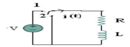
At t=0-, , switch k is kept at position 'a' for very long time. Thus, the network is in steady state. Initial current through inductor is given as,
