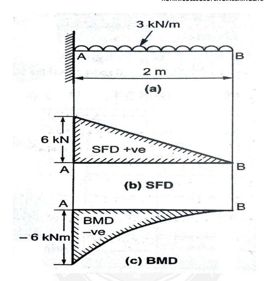
$\label{lem:bending-moment-calculation:} Bending moment Calculation: [Sum of (Vertical forcex Distance of load acting from required section)]$
