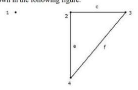
In this graph, the nodes 2, 3, and 4 are connected by two branches each. But, not even a single branch has been connected to the **node 1**. So, the node 1 becomes an **isolated node**. Hence, the above graph is an **unconnected graph**.
