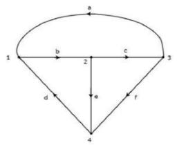
In the above graph, the direction of current flow is represented with an arrow in each branch. Hence, it is a **directed graph**.
