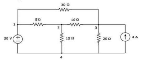
In the above circuit, there are **four principal nodes** and those are labelled with 1, 2, 3, and 4. There are **seven branches** in the above circuit, among which one branch contains a 20 V voltage source, another branch contains a 4 A current source and the remaining five branches contain resistors having resistances of  $30 \Omega$ ,  $5 \Omega$ ,  $10 \Omega$ ,  $10 \Omega$  and  $20 \Omega$  respectively.
