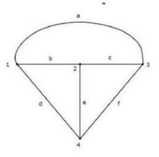
In the above graph, there are **four nodes** and those are labelled with 1, 2, 3 & 4 respectively. These are same as that of principal nodes in the electric circuit. There are **six branches** in the above graph and those are labelled with a, b, c, d, e & f respectively.
