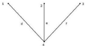
This connected subgraph contains all the four nodes of the given graph and there is no loop. Hence, it is a **Tree**. This Tree has only three branches out of six branches of given graph. Because, if we consider even single branch of the remaining branches of the graph, then there will be a loop in the above connected subgraph. Then, the resultant connected subgraph will not be a Tree.
