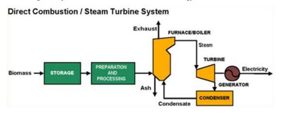
In a direct combustion system, processed biomass is the boiler fuel that produces steam to operate a steam turbine and generator to make electricity.
