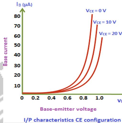
A curve is then drawn between input current  $I_B$  and input voltage  $V_{BE}$  at constant output voltage  $V_{CE}$  (0 volts).
