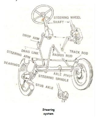
The steering system consists of many components, which are listed below:
