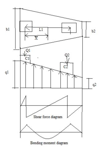
3.Design a trapezoidal footing for the two column shown in figure . Take allowable soil pressure is  $200 KN/m^2$ .
