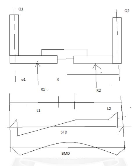
3. Design a strap footing for two columns with Centre to center distance 6.5m and distance between the reactions is 5.5 m. The allowable soil pressure is  $120\text{KN/m}^2$ .take eccentricity of footing of column is 1.The size of the column is 0.5mx0.5m
