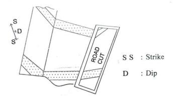
When there is no alternative in the above two undesirable cases, slope stability measures, such as perfect retaining wall, efficient drainage system etc, have to be taken before initiating the project.
