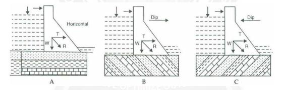
The most unfavourable strike direction is the one in which the beds strike parallel to the axis of the dam and the dip is downstream
