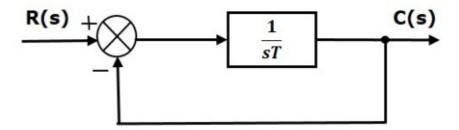
We know that the transfer function of the closed loop control system has unity negative feedback as,
