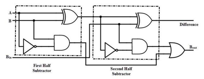
By comparing the adder and subtractor circuits and truth tables, we can observe that the output D in the full subtractor is exactly same as the output S of the full adder. And the only difference is that input variable A is complemented in the full subtractor.
