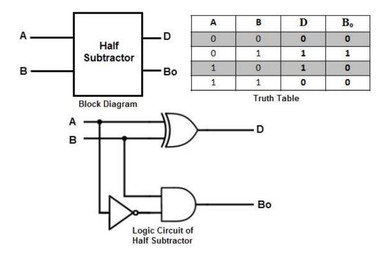
This circuit is similar to that of the Half Adder with only difference being the minuend input i.e., A is complemented before applied at the AND gate to implement the borrow output.
