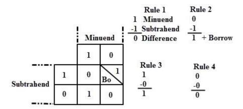
The above figure shows the four possible rules or elementary operations of the binary subtractions. In all the operations, each subtrahend bit is deducted from the minuend bit.
