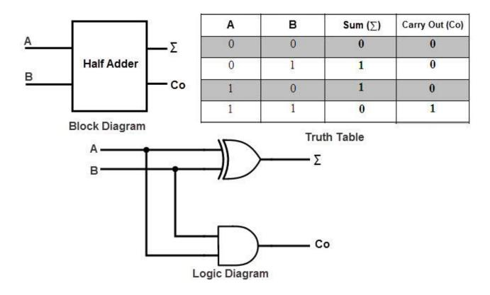
In the above half adder circuit, inputs are labeled as A and B. The 'Sum' output is labeled as summation symbol ( $\Sigma$ ) and the Carry output is labeled with C<sub>0</sub>.
